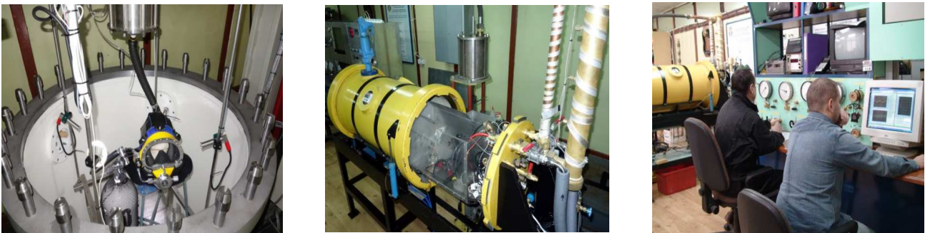
Fig. 5. The equipment of the Laboratory of Diving Apparatuses.
