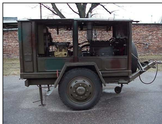
Fig. 4. The supply system for underwater works security base "ORTOLAN" with diving air compressors EK 2-150 manufactured by the USSR.
