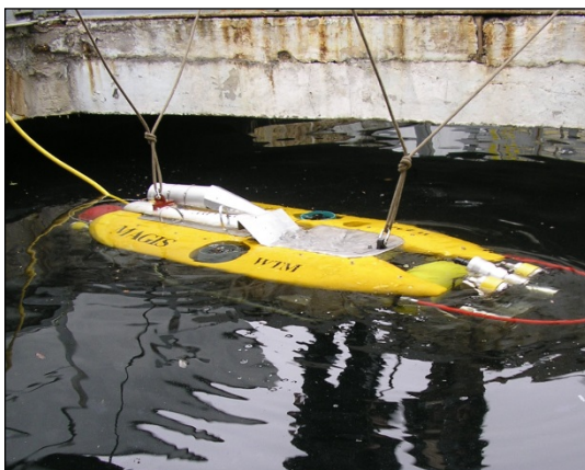
Fig. 8 Testing of the properties of the MAGIS underwater vehicle in the technological pool of the Ship Technology Department of the Szczecin University of Technology.
