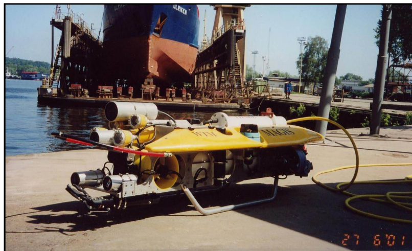
Fig. 7 The underwater vehicle MAGIS during technical condition surveys of the floating dock at the Szczecin Shiprepair Yard Gryfia.
