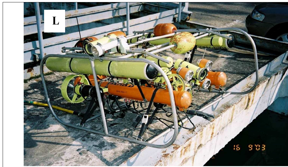
Fig. 3 Unmanned remotely operated underwater vehicle (ROV) KRAB II equipped with laser tracer L for the study of the vehicle's trajectory.
