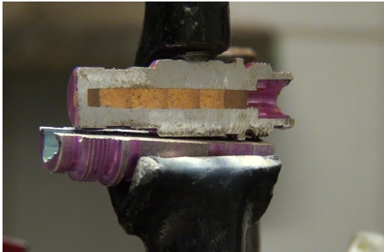
Photo 5. Test sample - longitudinally cut pyrotechnic retarder of an NGP-76 underwater rifle grenade, immediately before ignition by laser beam.
