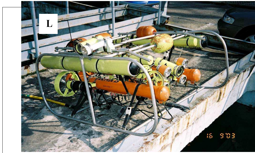
Fig. 3 Unmanned remotely operated underwater vehicle (ROV) KRAB II equipped with laser tracer L for the study of the vehicle's trajectory.
