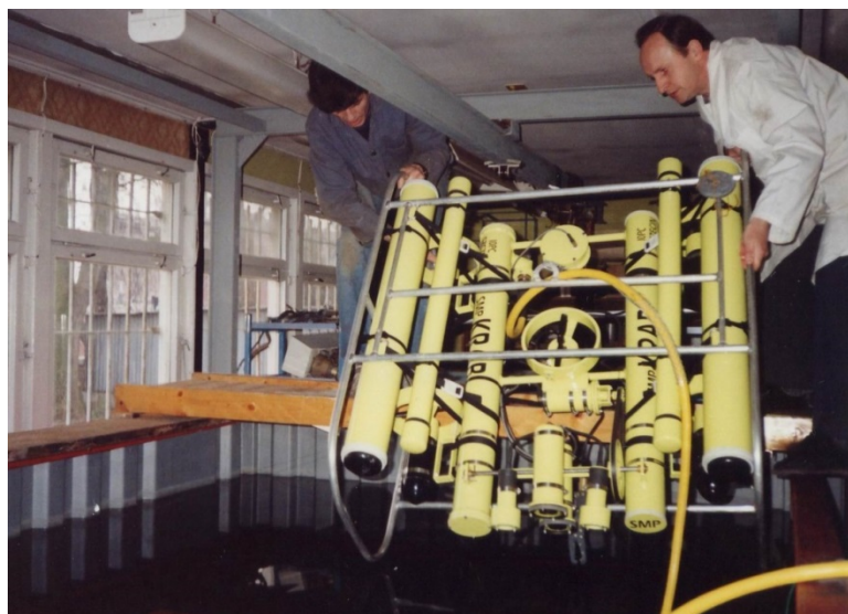
Fig. 2 KRAB I unmanned remotely operated underwater vehicle - first launch in the indoor technological basin of the Faculty of Marine Engineering of the Szczecin University of Technology.
