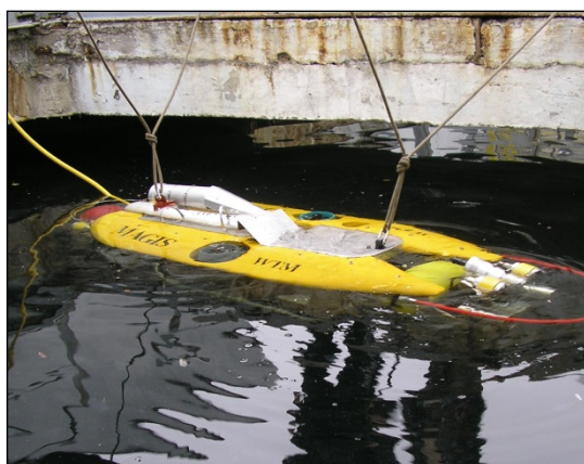
Fig. 8 Testing of the properties of the MAGIS underwater vehicle in the technological pool of the Ship Technology Department of the Szczecin University of Technology.
