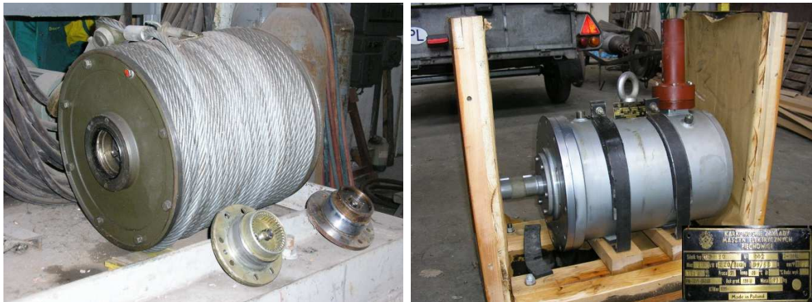
Fig. 4 The NUR work equipment carrier components: lift and electric motor of the drive system.
