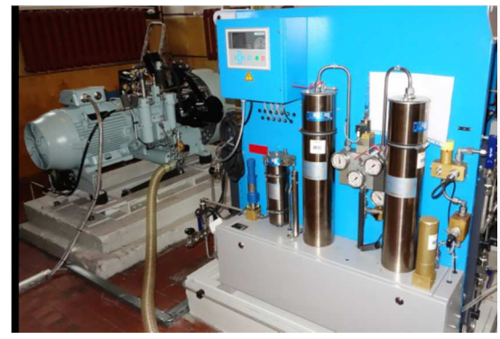
Fig.1-2 Configuration of the breathing air supply and treatment equipment of the DGKN – 120 complex. Source: own study.
